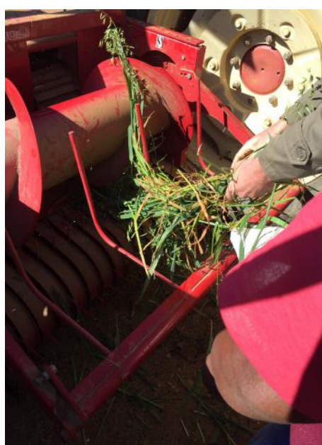
Figure 1 – Cutting the samples with the Ferraboli chopper
