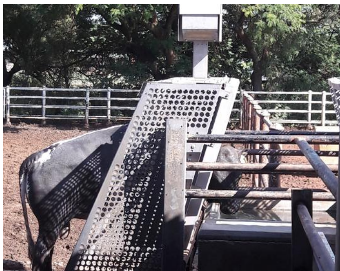
Figure 2 An animal is drinking water. Note that it is standing with its front legs on the scale and a partial body weight is taken. The antenna at the top transfers the information in real-time via radio link to the computer in the office (figure 1).
