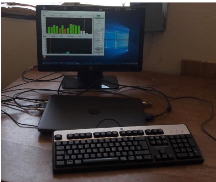
Figure 1 gives an indication of the real time recording of feed intake (Orange [animal present at feed bin] & Green bars [no animal present]) as well as partial body weight at water intake (Blue bar [animal present at water trough]).
